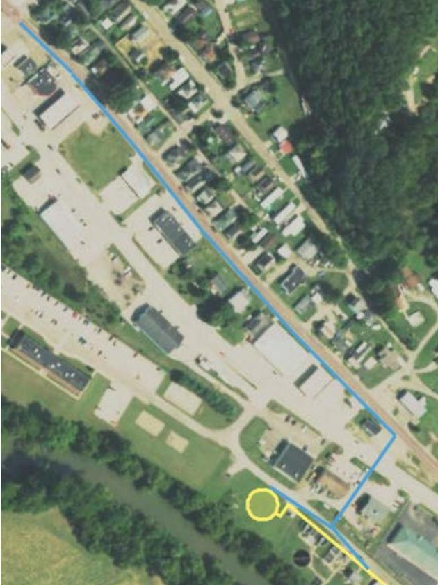
Figure 5 – Proposed lift station (yellow circle) and force main (yellow line) in Nelsonville
