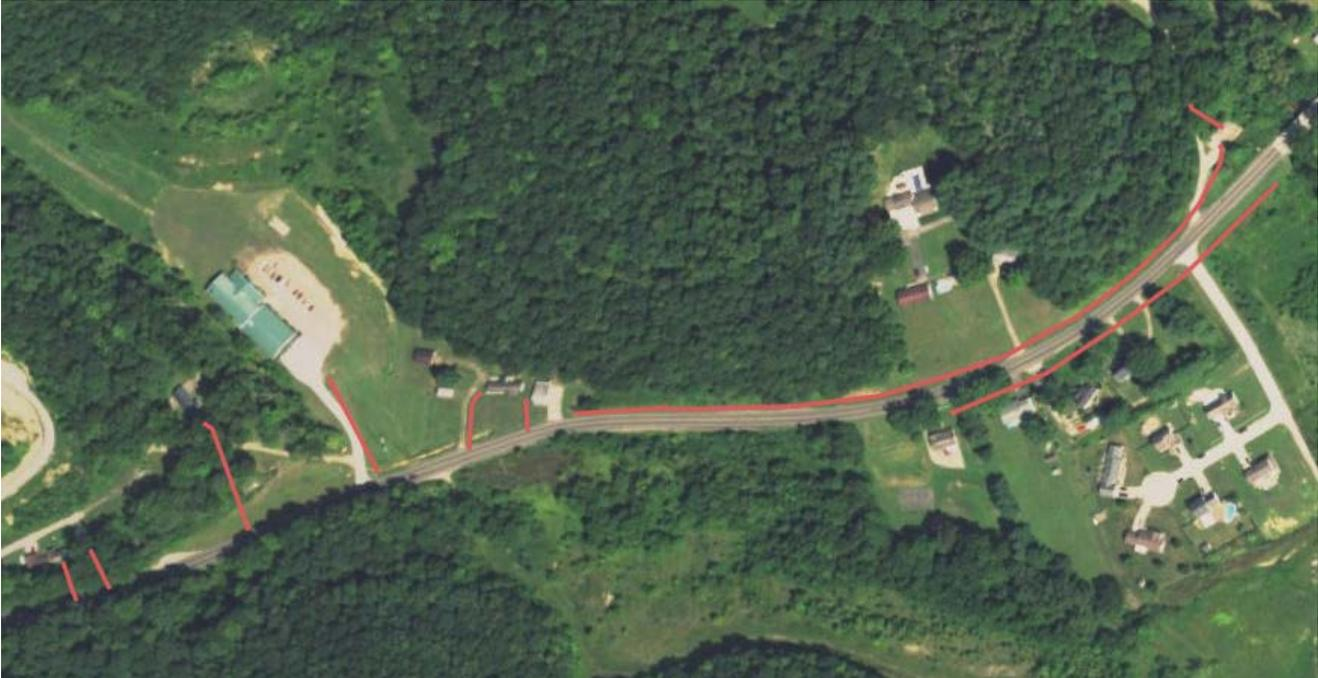
Figure 3 – Proposed gravity sewer along Carbon Hill Buchtel Road and Buchtel lift station (red box)
