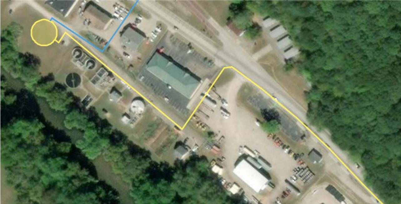
Figure 6 – Proposed force main (yellow line) along E. Canal /Old US 33 to site of new WWTP
